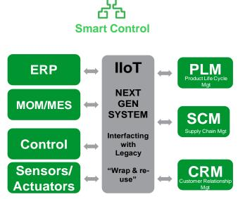
Next generation IIoT systems will allow better integration of legacy production, life-cycle and supply chain systems to improve overall enterprise efficiency & flexibility
